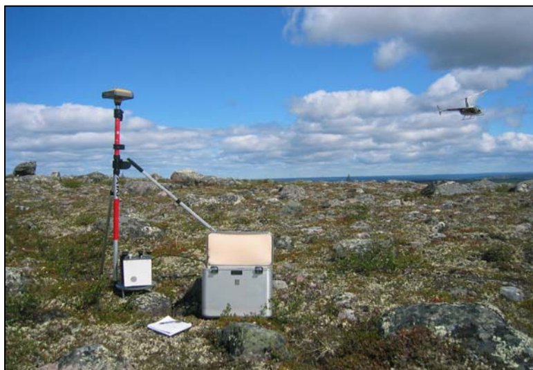
Figure 16: LaCoste & Romberg Gravity meter and TOPCON GPS receiver in field use.
