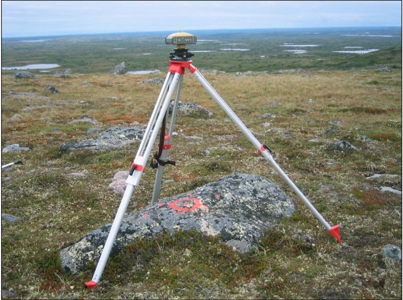
Figure 14: TOPCON HyperLite GPS receiver collecting data on GPS base station.
